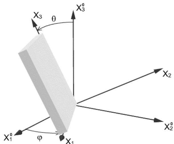
Figure 2:  $\phi$  and  $\theta$  cut angles
