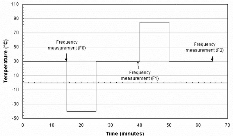
Figure 18: Temperature cycle
