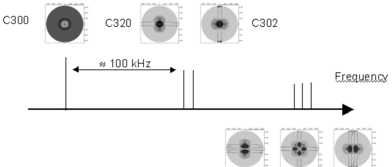
Figure 7 : Anharmonics of an SC-cut resonator on 3<sup>rd</sup> overtone
