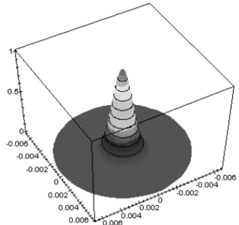
Figure 5: amplitude of vibration in the plate plan in a plano-convex resonator
