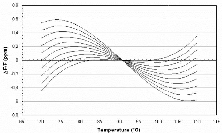
Figure 14: Frequency-Temperature characteristics of SC-cut for different values of  $\theta$
