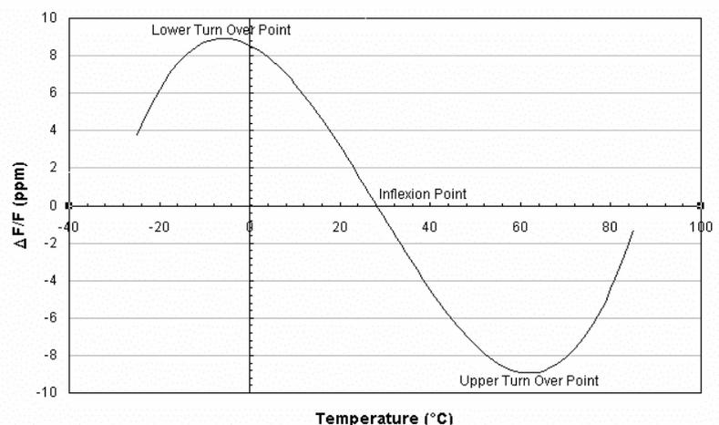
Figure 12: Typical frequency-temperature curve ( AT-cut )
