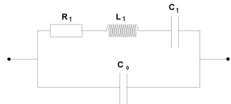
Figure 8: Equivalent electrical circuit
