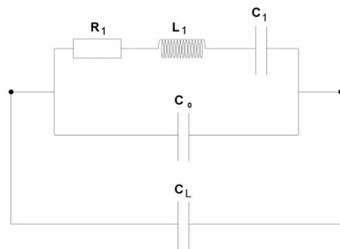
Figure 11: Load capacitance in parallel
