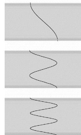
Figure 6: 1<sup>st</sup>, 3<sup>rd</sup> and 5<sup>th</sup> thickness shear overtones
