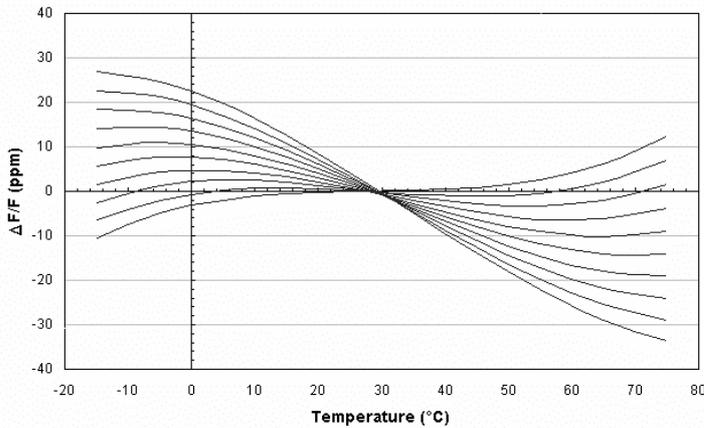
Figure 13: Frequency-Temperature characteristics of AT-cut for different values of  $\theta$
