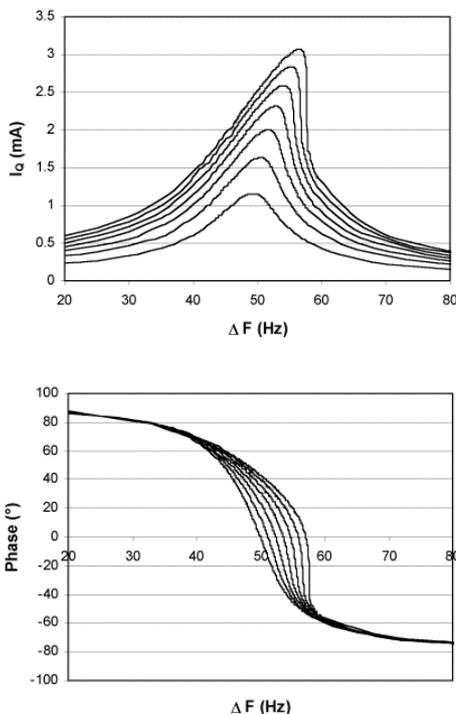
Figure 16: Resonance and phase curves for different drive levels
