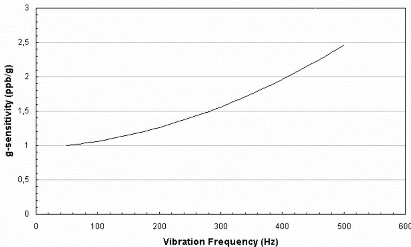
Figure 20: G-sensitivity vs vibration frequency
