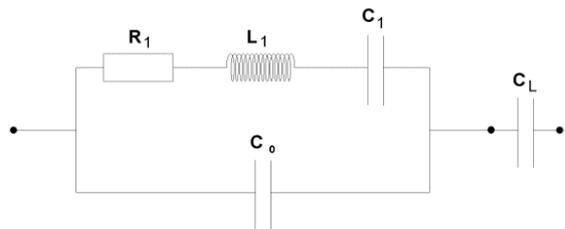
Figure 10: Load capacitance in series
