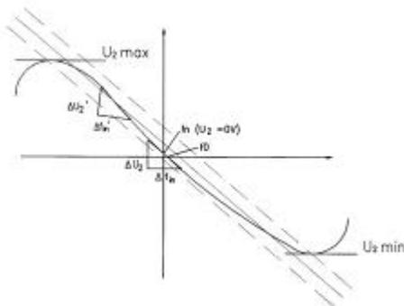
The non-linearity ( $\lambda$ ) of the voltage-frequency-characteristic is the percentage deviation of the output voltage  $U_2$  from a linear shape. Monolithic crystal discriminators are available for narrow-band FM combined with FM-demodulators.
