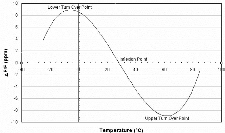
**Figure 3 Typical temperature characteristics of AT-cut crystals**
