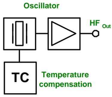
**Figure 2 Block diagram Temperature Controlled Crystal Oscillators**
