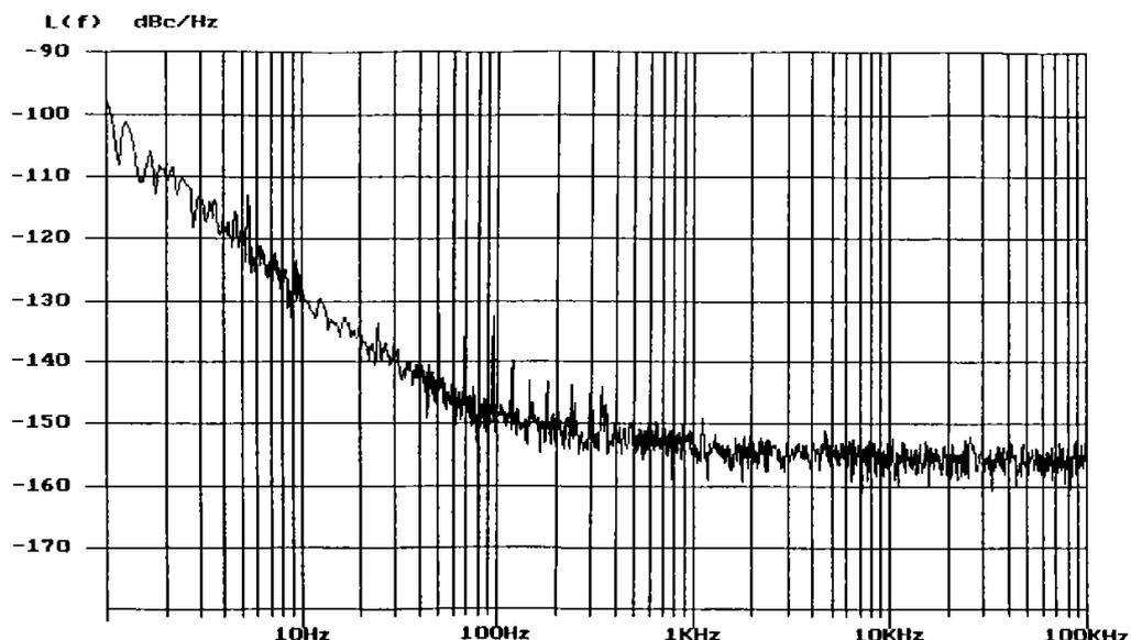
**Figure 5 Typical phase noise plot of a low noise crystal oscillator**
