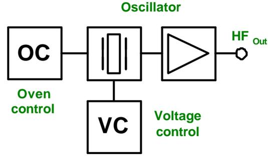
**Figure 4 Block diagram Temperature Controlled Crystal Oscillators**
