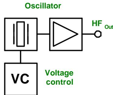
**Figure 2 Block diagram Voltage Controlled Crystal Oscillators**
