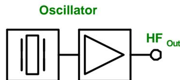
**Figure 1 Block diagram crystal oscillator**
